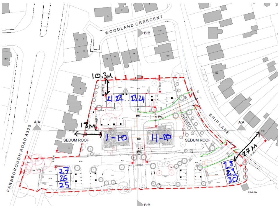
Figure 4: distance separation between units.
